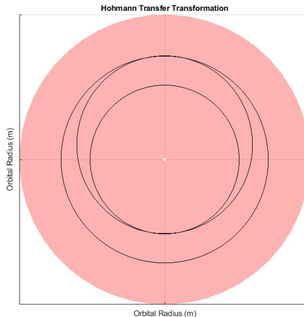
Figure 4-4 Hohmann Transfer Orbit, viewed from x-y perspective
